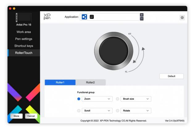
The driver enables zoom (default), brush size, scroll and rotate functions. Click the drop-down menu to customize roller functions.
