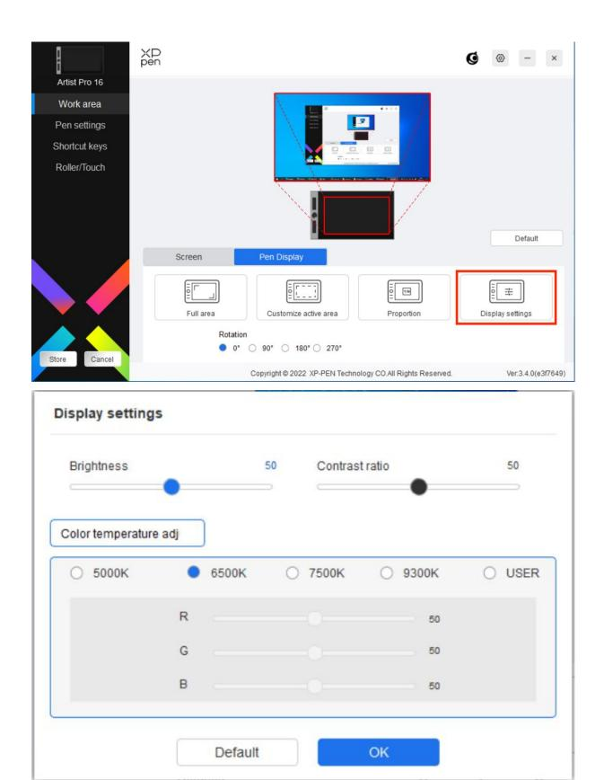
Color temperature: The driver enables five modes, i.e., 5000K, 6500K (default), 7500K, 9300K, and USER. In the USER mode, color temperature can be customized by adjusting the R, G and B values.
