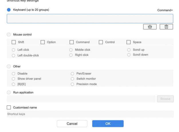
You can set a combination of multiple keys such as Ctrl+C and Ctrl+V. When you press the combination key, the set shortcut keys will all run once.
