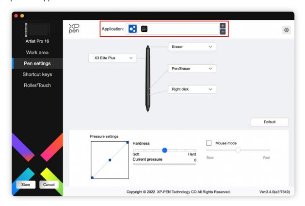
Select an application from the list of applications at the top of the driver, tick the application, and then customize its pen keys, shortcut keys and roller/touch functions.
