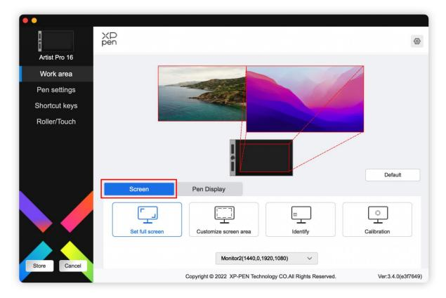
You can set the mapping between the display area of the current screen and the device.
